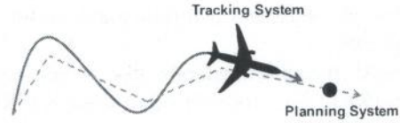
Fig. 1: A planning system using a fast but simple model, followed by a tracking system using a dynamic model
