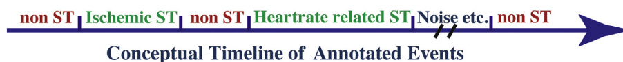
Fig. 1. Conceptual timeline of annotated events in the LTST database. Events marked in green form up the ST condition. Events marked in red represent the non-ST condition. Events marked by black include noise, unreadable segments and sudden ST shifts, which are removed from analysis. (For interpretation of the references to color in this figure legend, the reader is referred to the web version of this article.)
